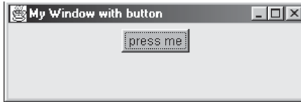
Figure 8.3 Adding a button to a window container
